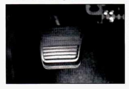
Hold the regular brake pedal down with your right foot. Push down the parking brake pedal with your left foot. If the ignition is on, the brake system warning light will come on.
